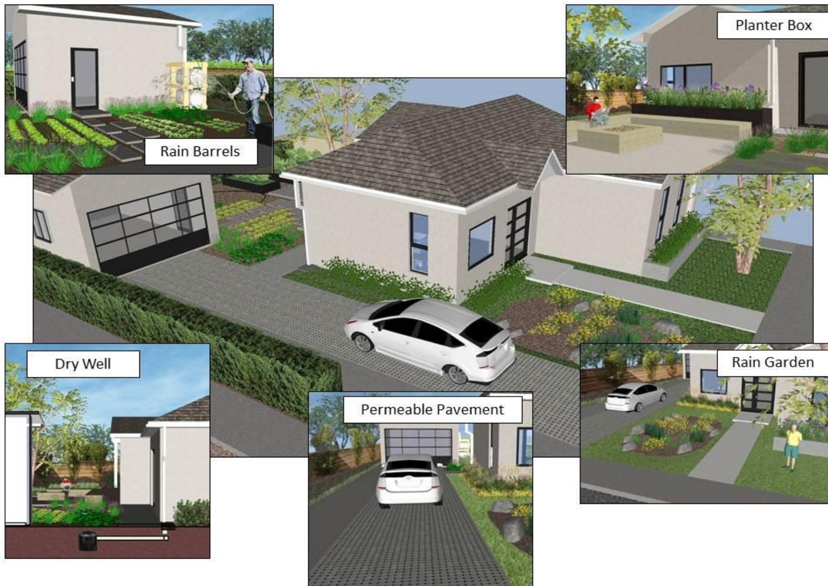
Figure 3.1- Small Scale Residential BMP Schematic
