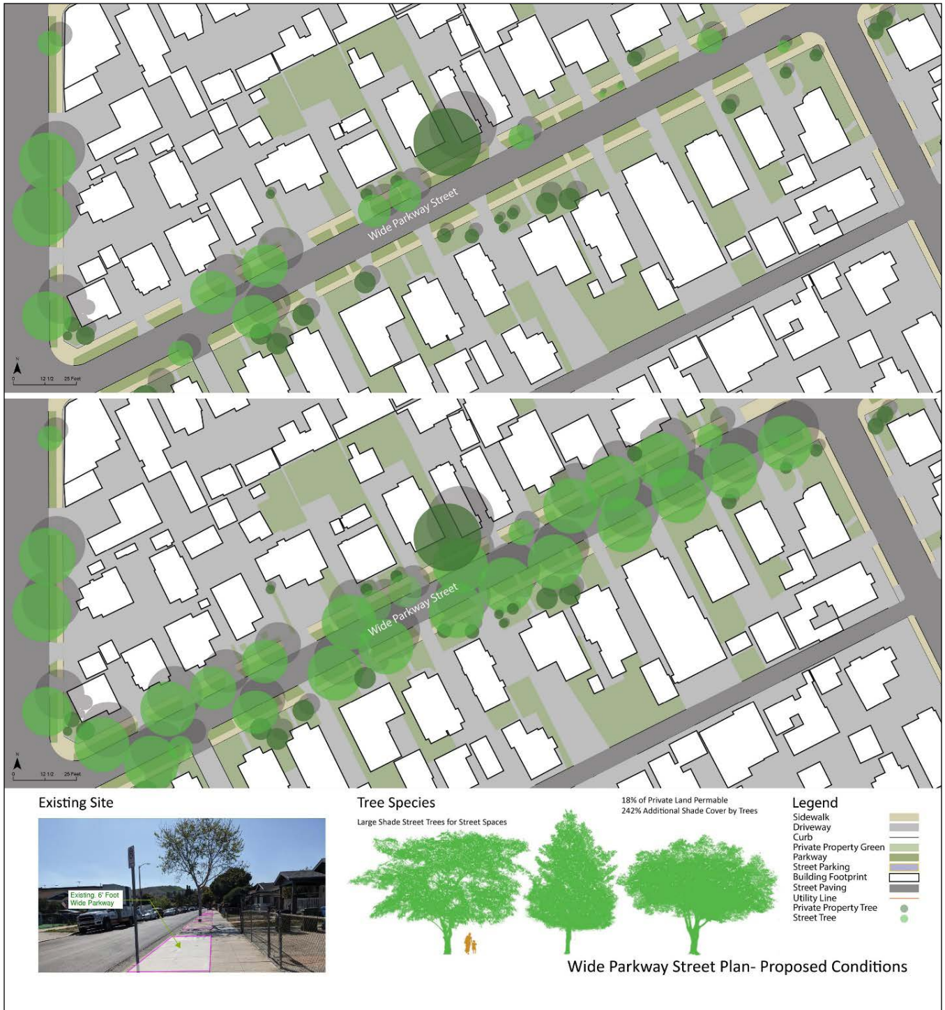
Figure 23: Potential tree planting vision for a street with a wide parkway showing the current (top panel) and potential tree cover (middle panel) and their shading potential with miscellaneous pictures and legend in lower panel
