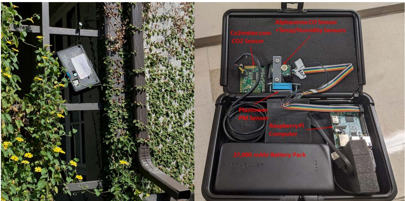
Figure 15: Sensor hanging from porch trellis (left) and components of portable sensor package (right)
