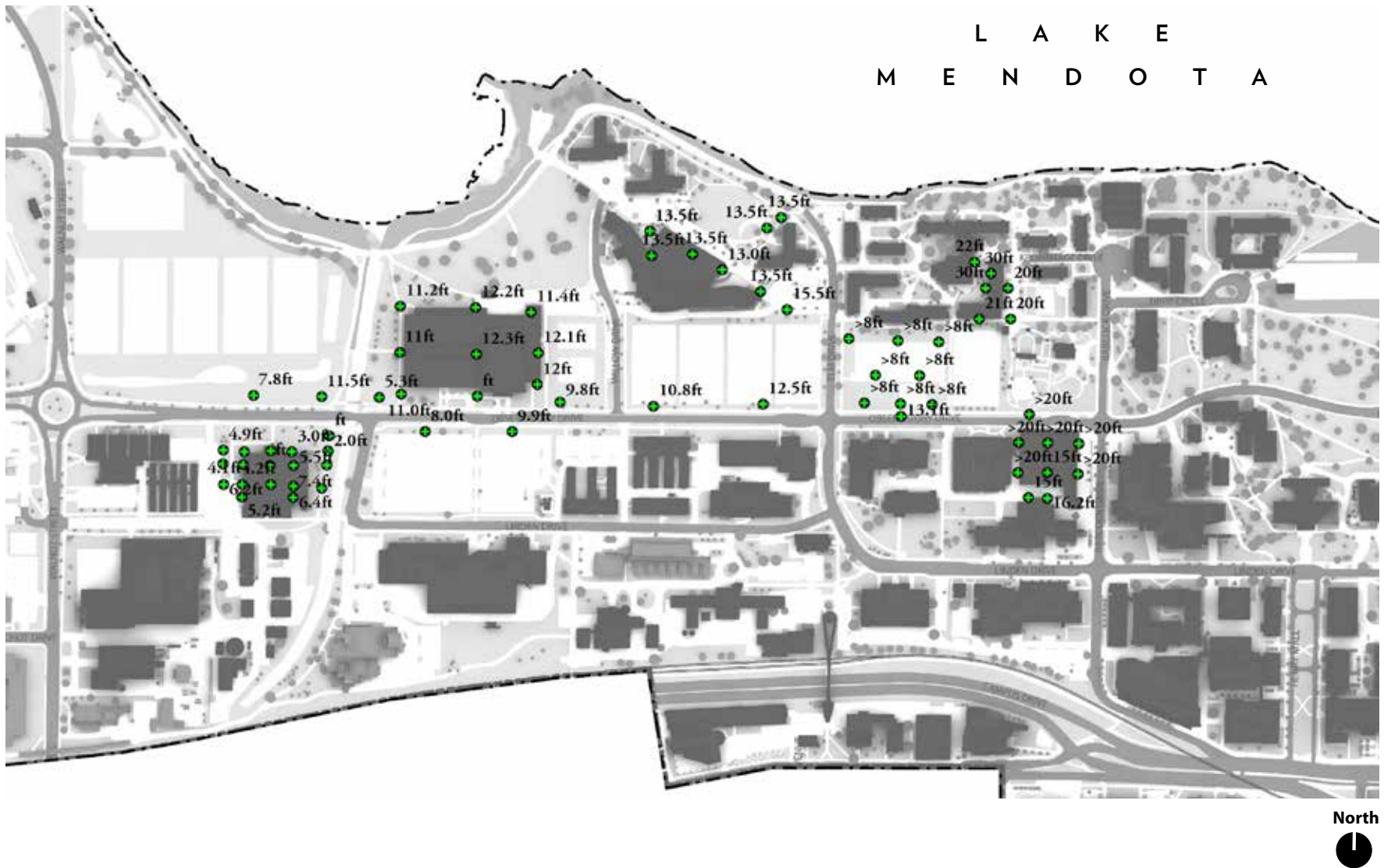
Figure 3-8 Groundwater Depths Per Soil Borings – Near East and Near West Campus
