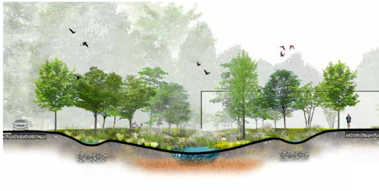
Figure 5-2 Cross Section Rendering of a Biofiltration Area With Wet Pool
