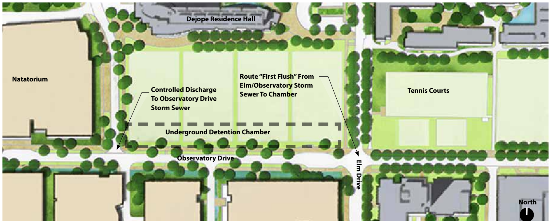
Figure 5-15 Close-Up of Underground Detention Chamber at Near East Recreation Fields
