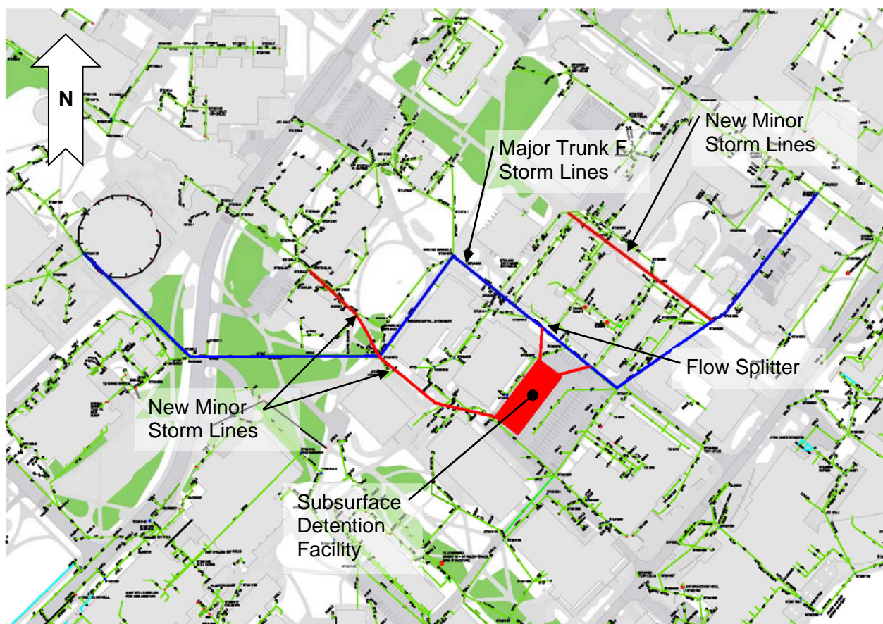
Figure 6.t. Recommended Improvements in the Trunk F Area
