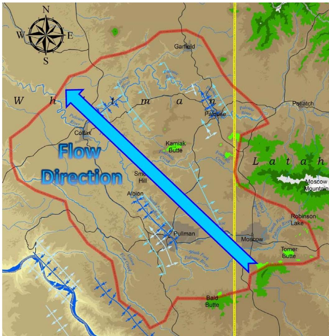
**Updated Figure 5. Conceptual Representation Ground Water Flow Direction in the lower aquifer in the Pullman-Moscow Basin**
