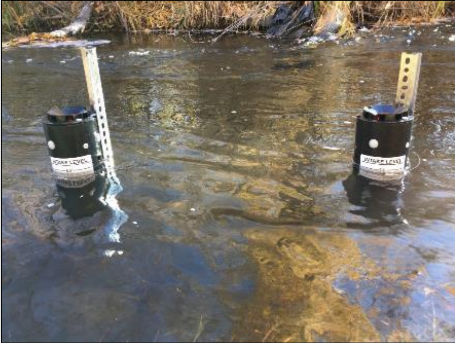
Image 8.0.1: In-stream sampling equipment
