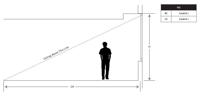
For Top-lighting Daylight Zone (see diagram below):
