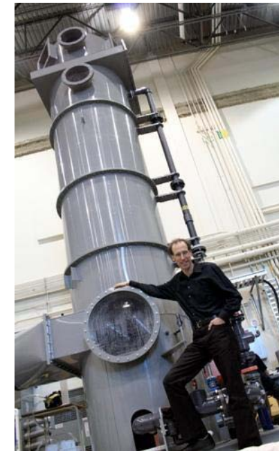
David Keith, University of Calgary climate change scientist stands by the machine he and his team are using to isolate carbon dioxide from the air. Credit: Image courtesy of University of Calgary, Sciencedaily.com
