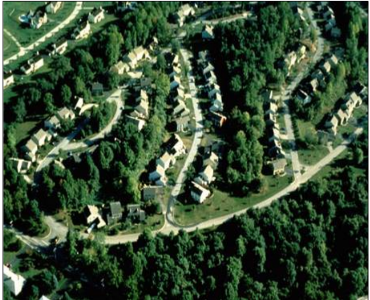
Figure 5.2 Aerial photograph of development project illustrating preservation of undisturbed natural areas (Source: Arendt, 1996)
