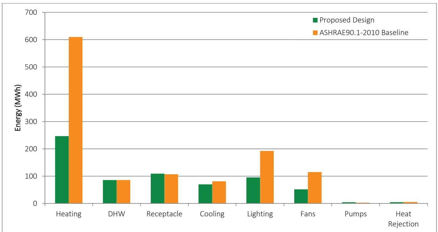
FIGURE 4: ANNUAL ENERGY CONSUMPTION IN EACH DESIGN OPTION AND BASELINE MODEL
