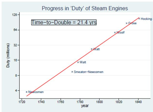
Figure 1: Increase in Duty of Steam Engine.
