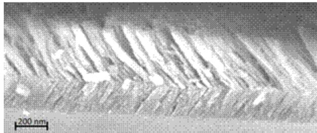
**Figure 2:** Cross-sectional scanning electron image of a multi-layered nanostructured of  $\text{SiO}_2$ .
