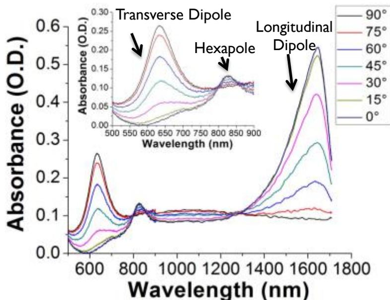
Figure 1: Plasmon spectra as a function of incident light polarization
