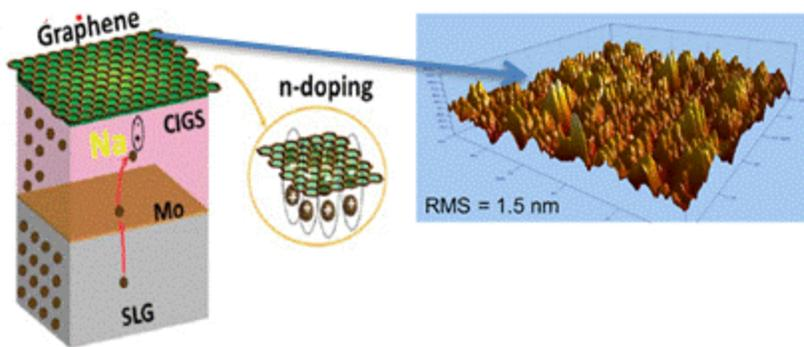
**Figure 1:** Eliminated the use of CdS as buffer layer and replaced it with graphene. The n-doping reaches  $2.11 \times 10^{13} \text{ e/cm}^2$  when graphene is transferred onto a p-type CIGS deposited onto soda lime glass.
