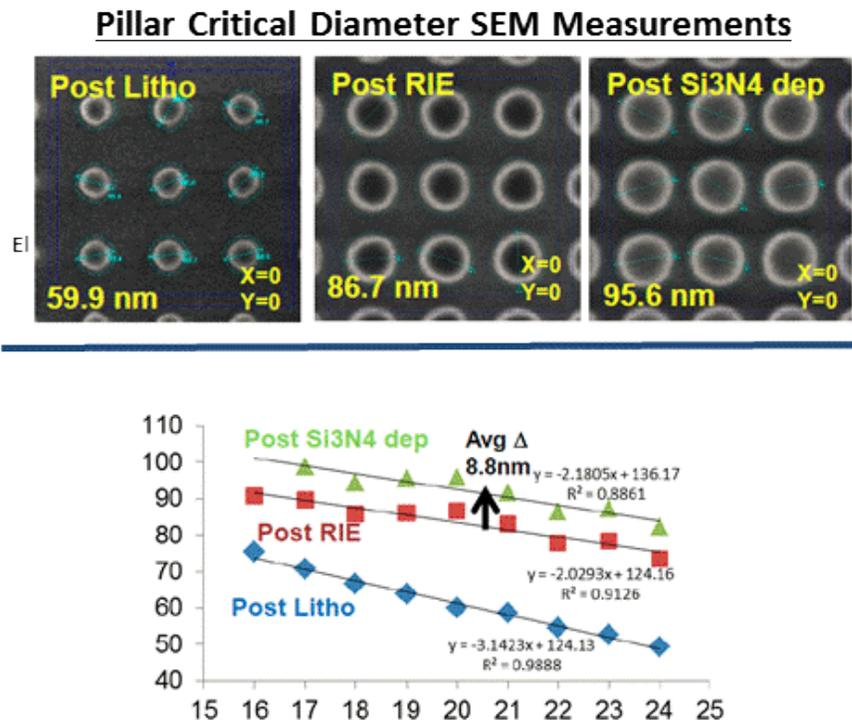
**Figure 1:** SEM micrographs illustrate how dual exposures created a 2D array of resist pillars of varying diameters. Towards the higher extreme of the lithographic process budget, the features began to coalesce into each other. The diameter of the ARC pillars post RIE was measured as a function of dose for each of the nine areas.
