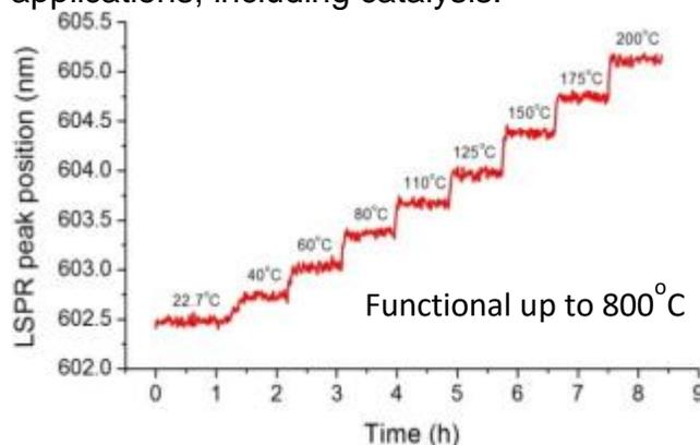
Figure 3: Plasmon peak position as a function of temperature
