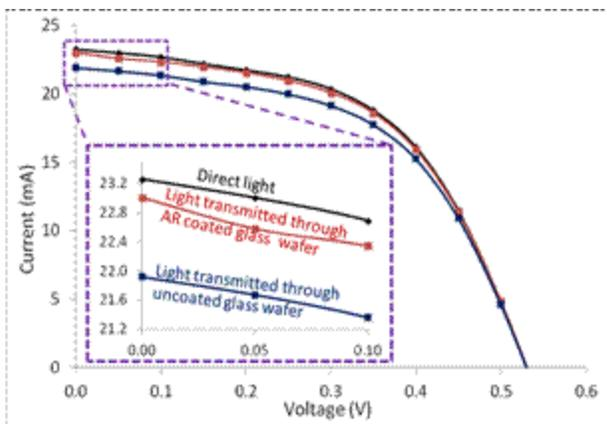
**Figure 3:** Current-voltage characteristics of a CIGS photovoltaic device under illumination of direct light, as well as light transmitted through an AR-coated glass wafer and light transmitted through an uncoated glass wafer.
