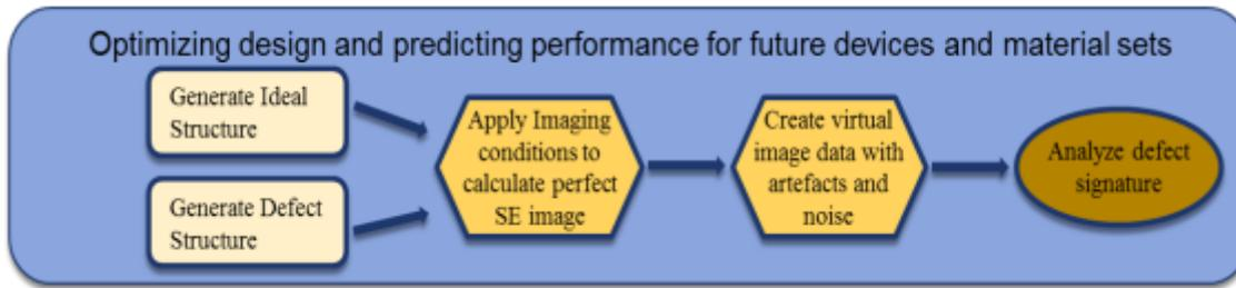
**Figure 3:** Flowchart for virtual image data generation.
