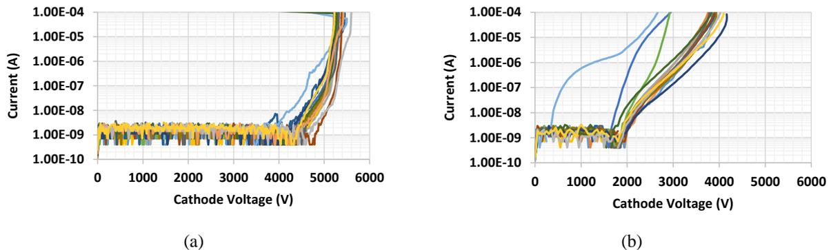
Fig. 16: Blocking behaviors of randomly selected 16-PiN diodes with (a) Hybrid-JTE, dose= $1.8 \times 10^{13} \text{cm}^{-2}$ , (b) 35-FFR.
