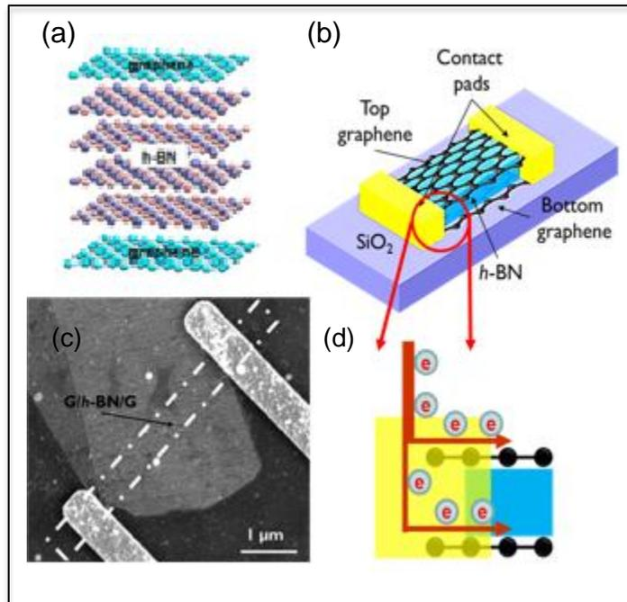
**Figure 2: Carbon-based Interconnects.** (a) Atomic-lattice schematic of a double-layered graphene (DLG) heterostructure separated by an interposing h-BN multilayer; (b) SEM image showing the heterostructure with two probing contacts. Here, the dash-dotted lines show the edges of plasma-etched graphene ribbon for eye-guiding purpose. (c) Schematic tilted-view of the DLG structure. (d) Zoomed-in view showing the detail of graphene-metal contact.
