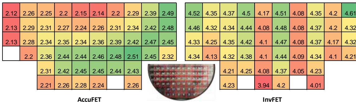
Fig. 9. Distribution of threshold voltages of SiC AccuFETs and InvFETs fabricated on 6-inch SiC wafers. A half-cut picture of a fully processed 6-inch wafer is also shown in the middle. Threshold voltages of AccuFETs show radial pattern across the wafer while those of InvFETs show random distribution.
