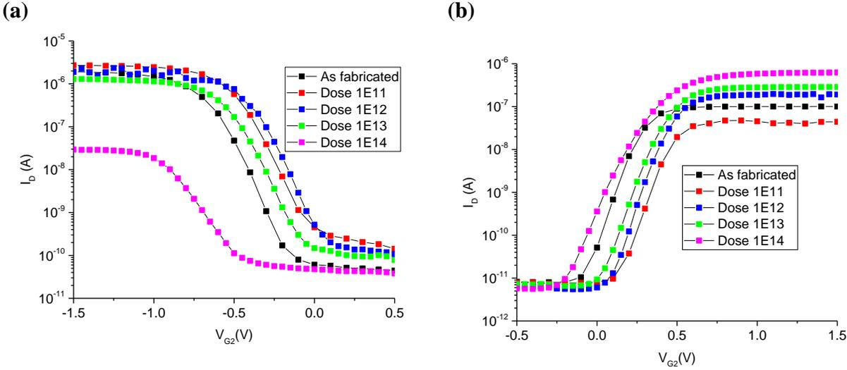
Transfer curves from a single reconfigurable MOSFET device under proton radiation. The device is fabricated using a 2D TMD WSe2 and can reconfigure into both p- and n-channel MOSFETs.
