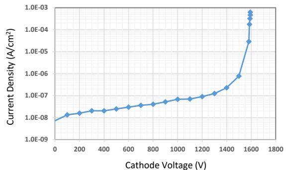
Fig. 6. Typical reverse characteristics of fabricated PiN diodes with Bevel-JTE measured after  $\text{N}_2\text{O}$  RTA process. Implanted JTE dose is  $1 \times 10^{13} \text{cm}^{-2}$ .
