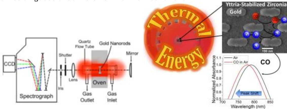
Figure 2: a) Schematic of the thermal imaging bench setup (left). b) Diagram showing the placement of the sample in the Macor holder inside the furnace (right). Interfacial surface reactions between CO and oxygen species are also shown.
