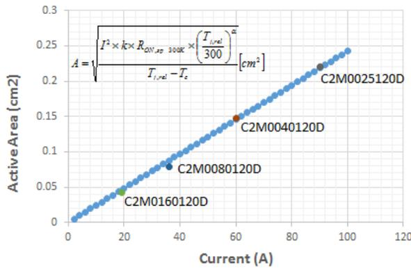
Fig. 1: Active area to target specific currents based on the proposed model (inset). Commercial 1200V SiC MOSFET information are also plotted, and well matched with the model.
