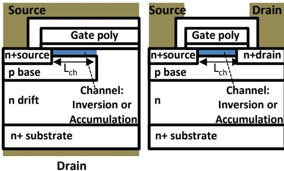
Fig. 7: Cross-sectional views of fabricated SiC Inversion mode and Accumulation mode MOSFETs ( $L_{ch}=0.5\mu\text{m}$ ), and lateral MOSFET ( $L_{ch}=200\mu\text{m}$ )
