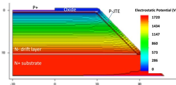
Fig. 5. Potential contour of Bevel-JTE at 1720V. JTE dose in this simulation is  $1 \times 10^{13} \text{cm}^{-2}$ .
