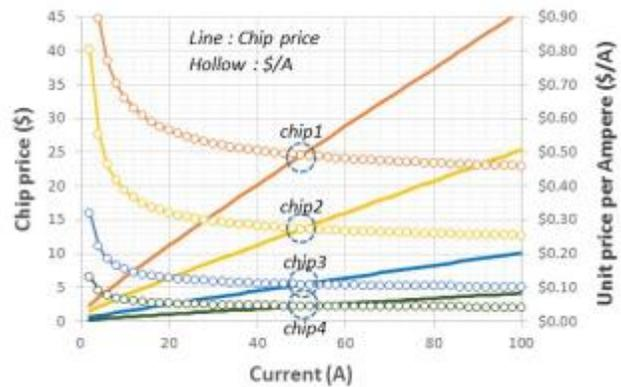
Fig. 2: 1200V SiC MOSFET price projection. Conditions in Table 1 were used in this analysis.
