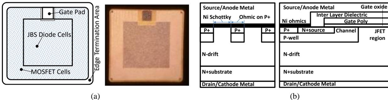
Fig. 13: (a) Schematic diagram of JBSFET layout and the chip image and (b) Cross-sectional view of JBS diode cell structure (left) and MOSFET cell structure (right). It is important to note that a single process, multi-purpose Ni contacts on 4H-SiC was used. The Schottky width is 4 μm and the cell pitch for the MOSFET is 11 μm with the channel length of 0.8 μm.
