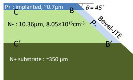
Fig. 4: Cross-sectional view of Bevel-JTE. JTE width for the conventional single-zone JTE is 50 μm, while that of Bevel-JTE is about 15 μm.
