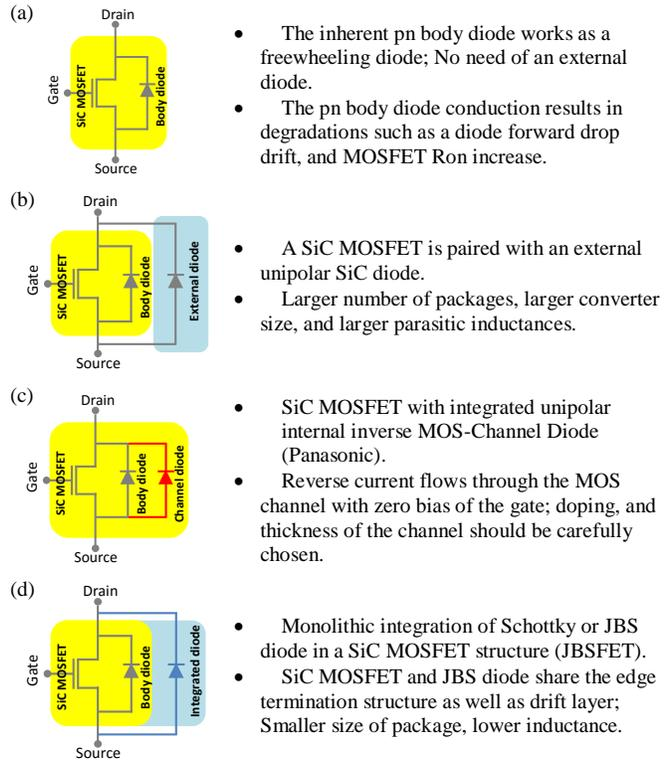
Fig. 12: Various approaches to accomplish SiC MOSFET and diode pair in a power converter application.
