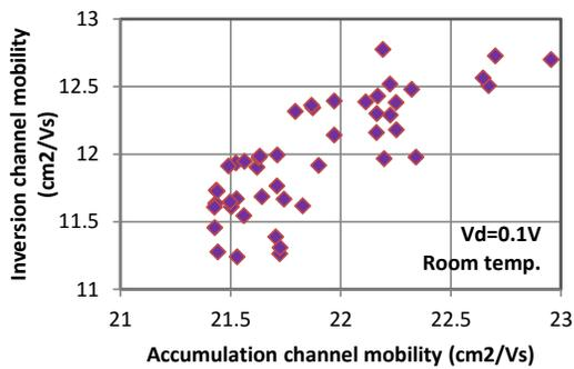
Fig. 10: Field effect channel mobilities extracted from  $I_d$ - $V_g$  of 52- lateral MOSFETs.  $L_{ch}$ =200  $\mu\text{m}$ , Channel width=200  $\mu\text{m}$ .  $V_d$ =0.1V,  $V_g$ =20V.
