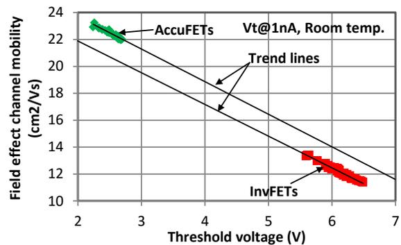
Fig. 11: Trade-off between channel mobility and threshold voltages. All data were measured from lateral MOSFETs. Channel designs and gate oxidation processes determine this trade-off.
