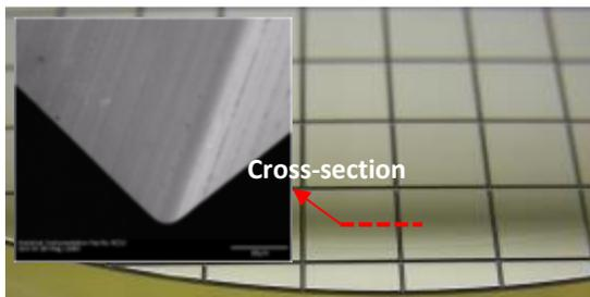
Fig. 3: Wafer image after bevel dicing. Scanning Electron Microscope (SEM) image of bevel surface with 45 degree blade is also shown.
