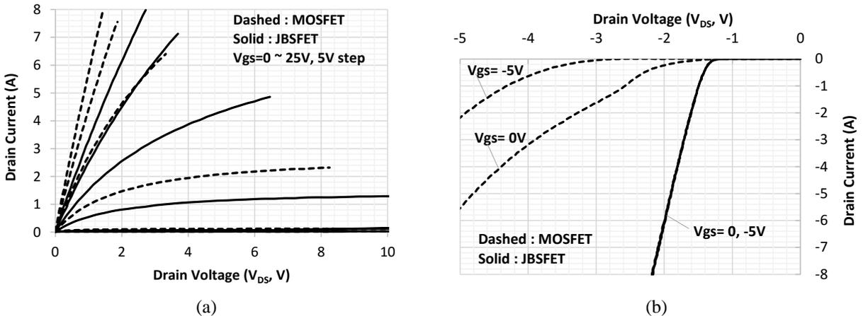
Fig. 14. Comparison of (a) the first and (b) third quadrant behaviors of the fabricated JBSFET and MOSFET. The JBSFET was annealed at 900°C for 2 minutes while the MOSFET was annealed at 950°C for 2 minutes. Both JBSFET and MOSFET have the same active area: 4.5 mm<sup>2</sup>. But, in the JBSFET layout, only 45 % of the active area was allocated for the MOSFET cells. Threshold voltages for both devices are the same: 2.7V at  $I_d=1$  mA. All data were measured on wafer at room temperature.
