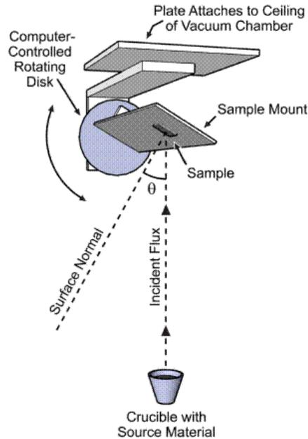
**Figure 1:** Illustration of the experimental setup used in the oblique-angle deposition technique for porous nanostructured materials. The incident physical vapor flux strikes the sample at an angle relative to the surface normal.
