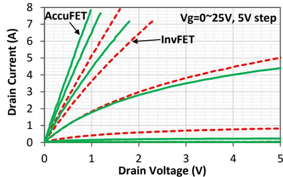
Fig. 8: Typical output characteristics of fabricated SiC AccuFETs and InvFETs. Active area:  $4.5 \text{ mm}^2$ , measured at room temperature.
