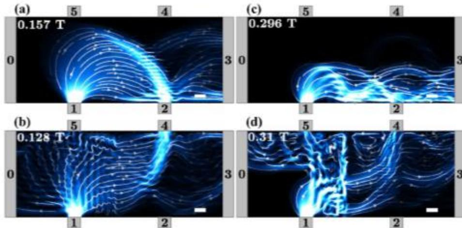
Modeling of electron trajectories in different magnetic fields for a unipolar (a) and (c), and an ambipolar (b) and (d) graphene devices.
