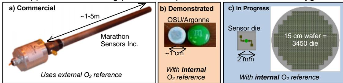
Figure 4: Comparison of scale and designs of industrially available O<sub>2</sub> sensors with the proposed design
