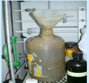
Improperly stored container: not labeled, open, in a sink
