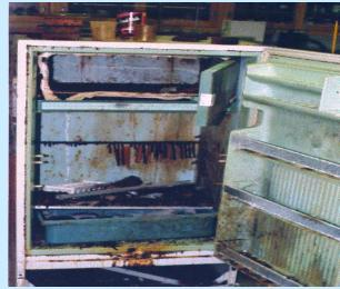
Flammable liquids stored in this non-explosion-proof refrigerator caused it to explode.
