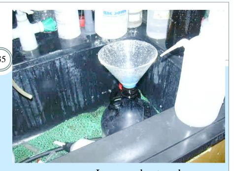
Improperly stored chemical waste. No secondary containment and open containers.
