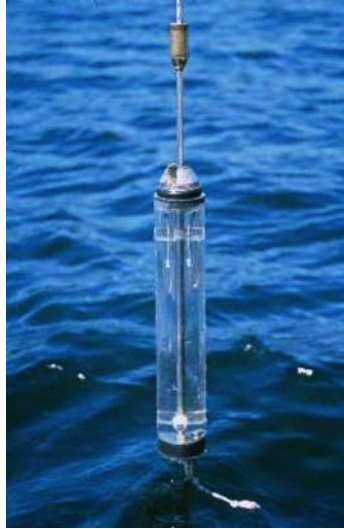
Figure 1. A Kemmerer sampler after it has been triggered by the messenger. [2]
