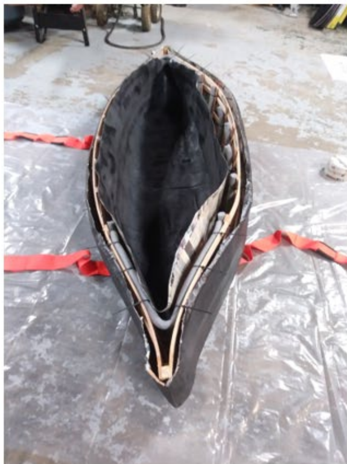
Above: The two molds and inner frame before being filled with spawn.
