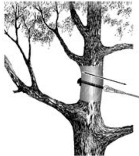
Fig. 33.5.3 Correct cable and hardware alignment
