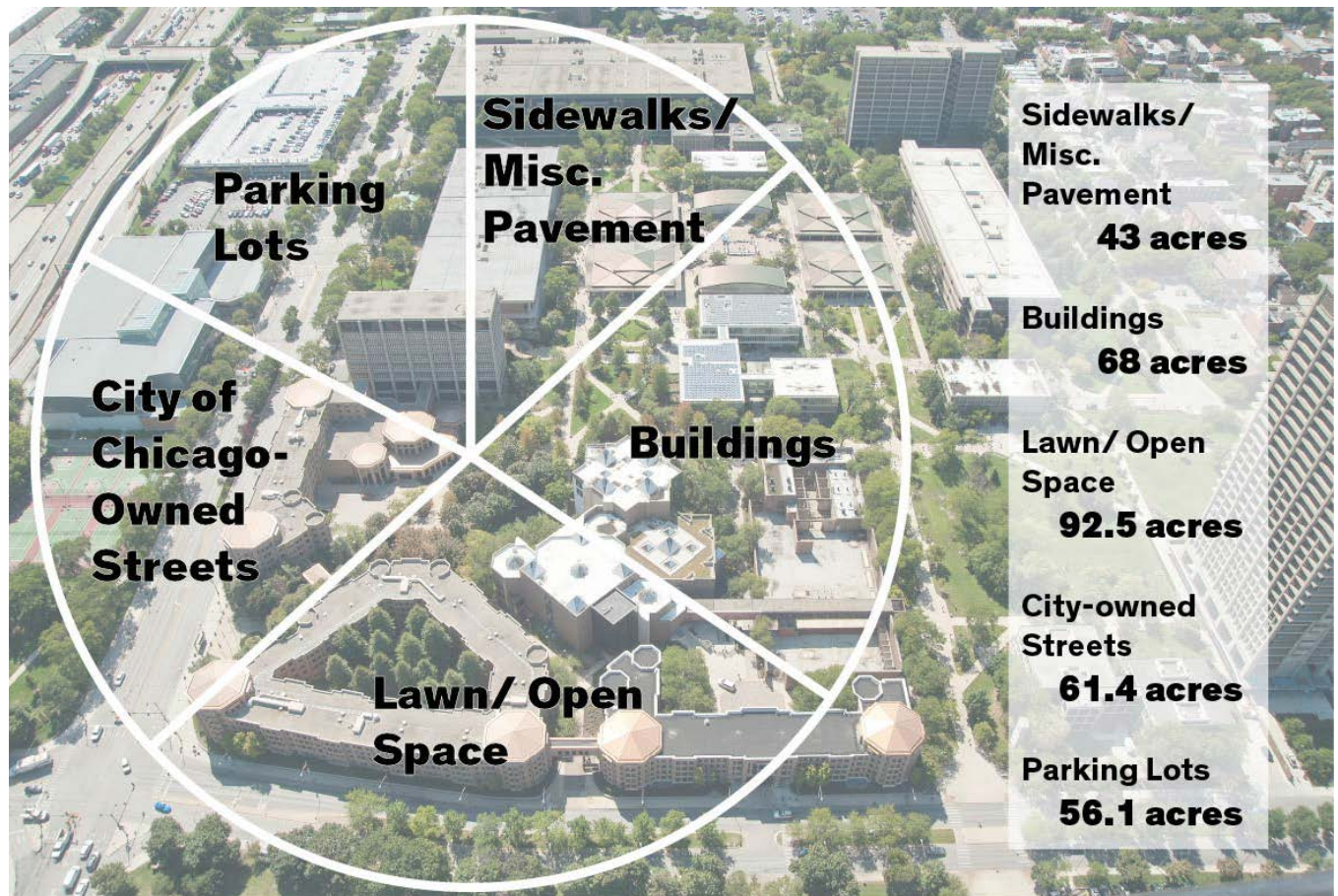
Figure 2. Existing (2018) land cover conditions (in acres) as calculated by land use GIS data layers from the University, the City of Chicago, and other regional sources.
