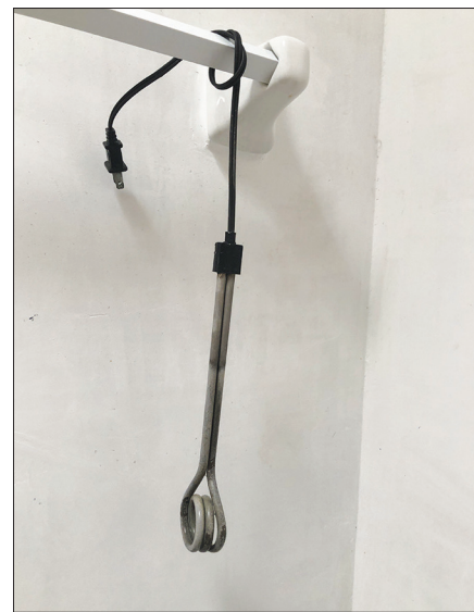
The hot-water heater, which is submerged into a bucket of water and plugged into the wall, is stored hanging on a towel rack when not in use.
