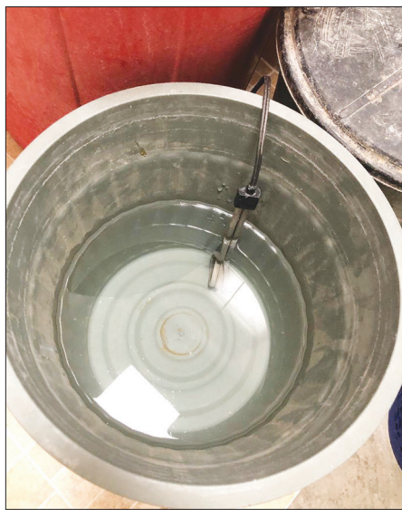
To heat water for bathing, just put this metal coil into the water bucket, and plug it into the outlet.
