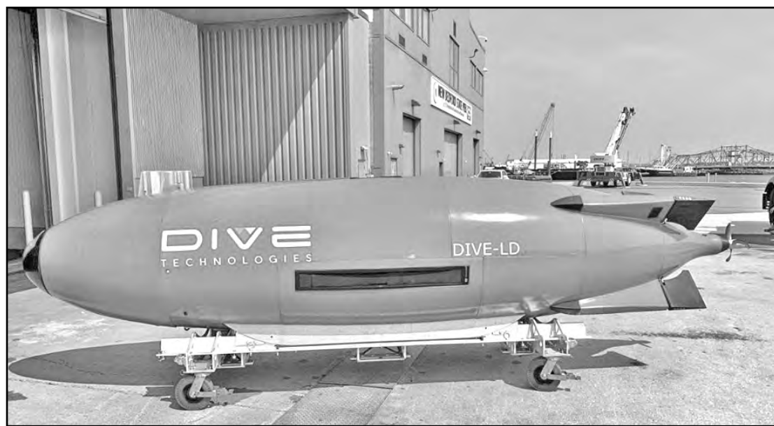
Virginia Tech ocean engineering researchers and students have supported the mission of Dive Technologies through development and testing of the DIVE-LD autonomous underwater vehicle, pictured above, which exceeded performance expectations at the first round of sea trials in Massachusetts in late 2020. Photo courtesy of Dive Technologies Inc.
