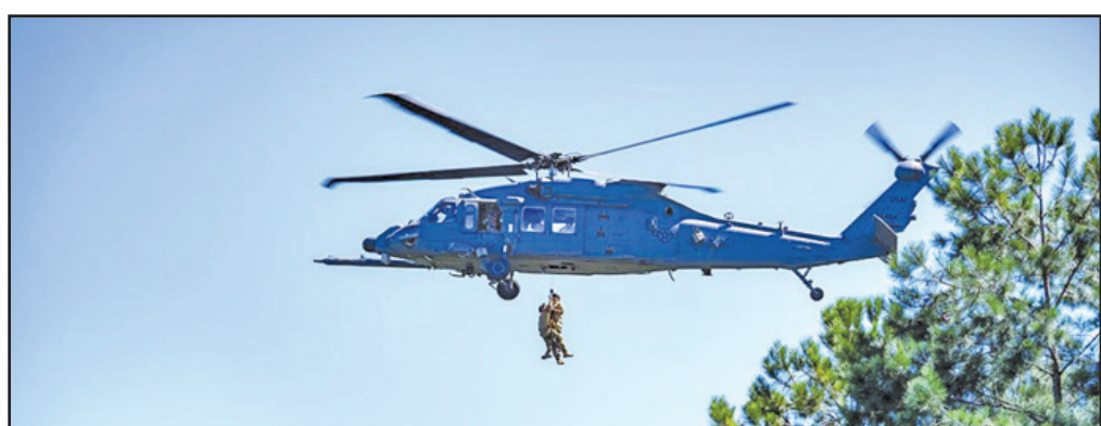
A U.S. Air Force HH-60W Jolly Green II from the 41st Rescue Squadron hoists pararescuemen during training at Moody Air Force Base, Georgia, in September. U.S. Air Force photo by Staff Sgt. Melanie A. Bulow-Gonterman.
