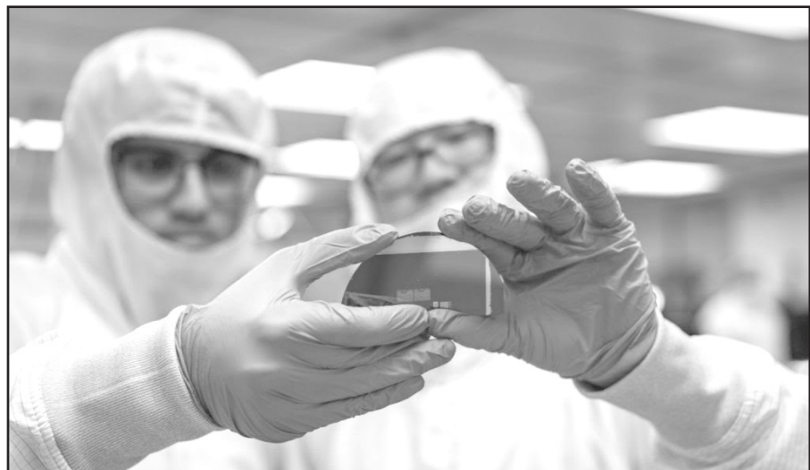
PHOTO BY LUKE HAYES FOR VIRGINIA TECH Students in the College of Engineering fabricate semiconductors in a clean lab. The lab uses a special yellow UV light and enhanced air filtration systems.
