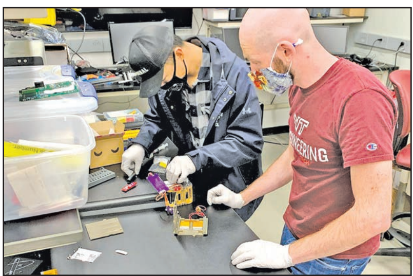
Students at Space@VT finalize assembly of their ThickSat, which will test a carbon fiber mast boom in low Earth orbit.
