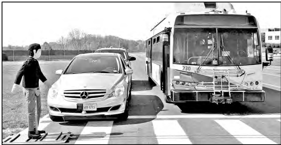
A robotic pedestrian used for sensor testing gets ready to cross a street on the Virginia Smart Roads.
