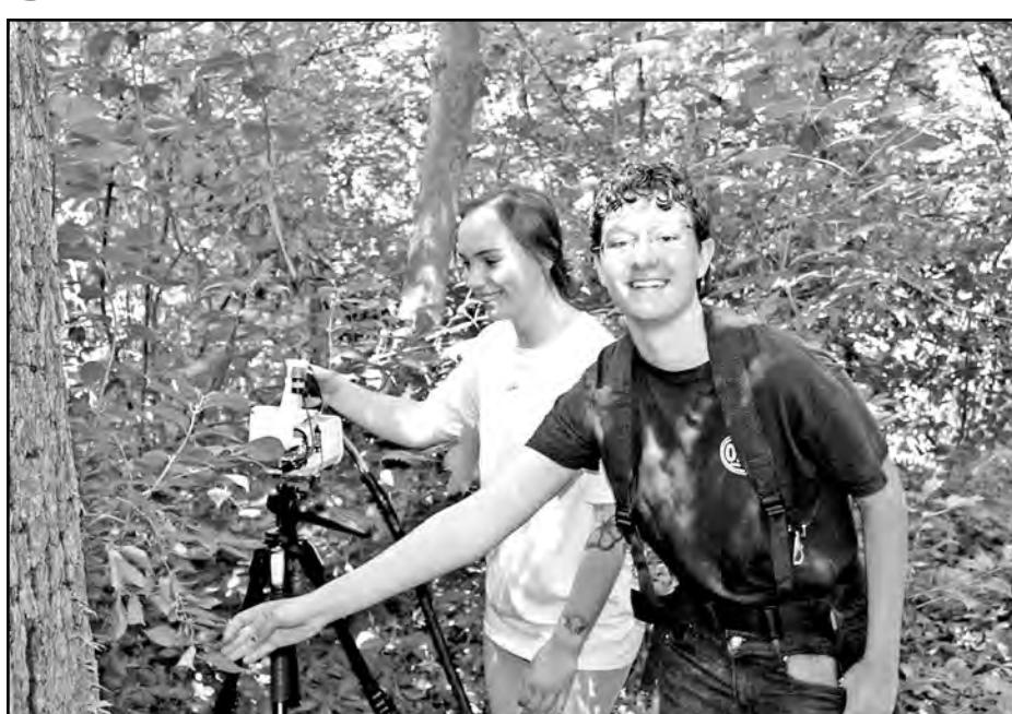
Abby Tenney (right) and Lesley Merkel (left) use a portable photosynthesis system to measure photosynthesis at different light levels on invasive and native plants in Stadium Woods. Photo by Helen Thompson.
