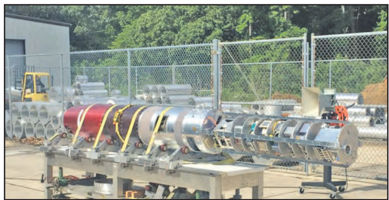
The payload section containing the eight RockSat-X undergraduate projects, prior to being incorporated into the Terrier-Improved Malemute sounding rocket. Photo courtesy of Abby Schefer, student manager of the national RockSat-X program.
