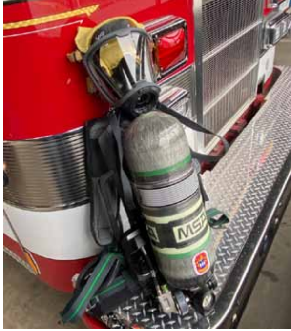
Nothing is more important for a firefighter's protection than the self-contained breathing apparatus. Pictured here is one of ten new airpacks purchased by SVFD. Not only do they protect firefighters, but also provide them with greater situational awareness including hot-spot tracking.
