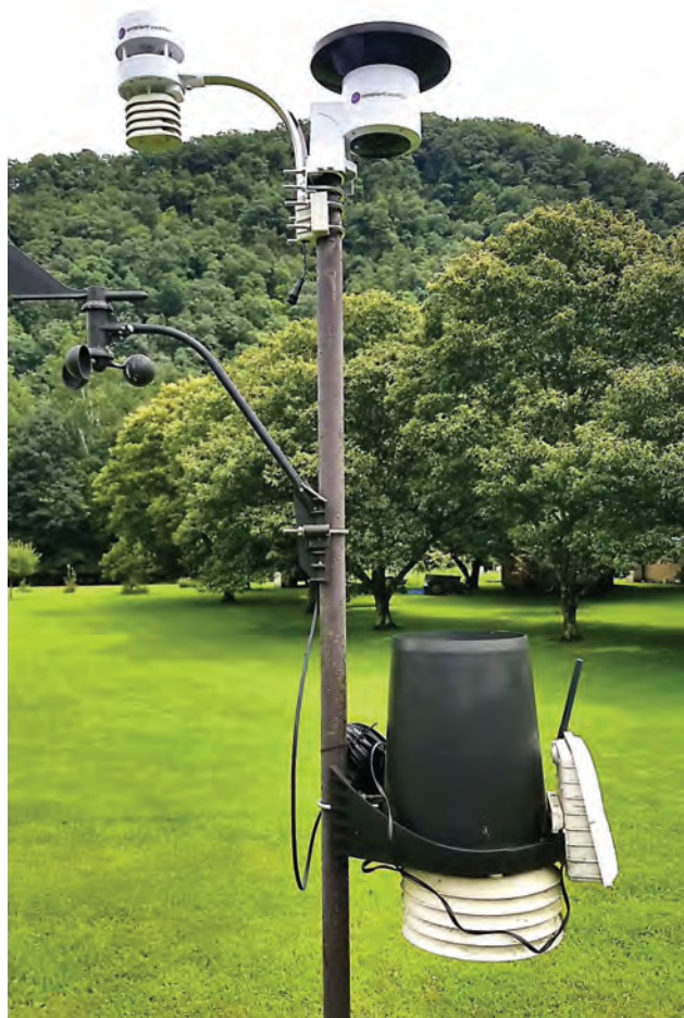
Dennis Filler's newly upgraded personal weather station with equipment from Ambient Weather (top) replacing the outdated equipment by Davis (bottom).
