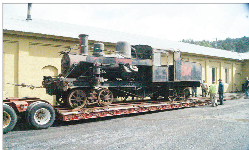
A Heisler Two Truck Steam Locomotive once owned by Stuart Thayer of Thomas is loaded onto a flatbed trailer to head to its new home in the Cass Collection at Cass Scenic Railroad.
