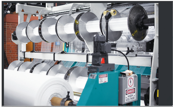
Apex Mills manufactures technical fabrics such as warp and circular knits, mesh/netting, elastomeric, and 3D spacer fabrics. Pictured above are warp knitting machines manufacturing 3D Spacer fabrics.
