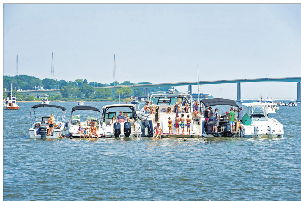
Docking, anchoring, or rafting within 20 feet of boats running generators or engines increases the chances of carbon monoxide poisoning and possibly even death. (Photos by Stacey Nedrow-Wigmore/BoatUS)
