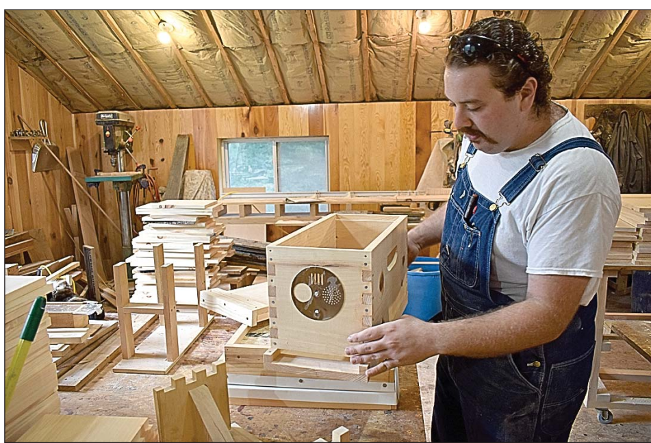
DUNMORE RESIDENT AND owner/operator of Lucas Millworks LLC, Lucas Prisco, assembles a nuc box, which is one of the honey bee products he creates. Nuc boxes are used to transfer bees, capture swarms and as queen rearing boxes. Prisco also makes bee hive boxes for collecting honey. S. Stewart photo
