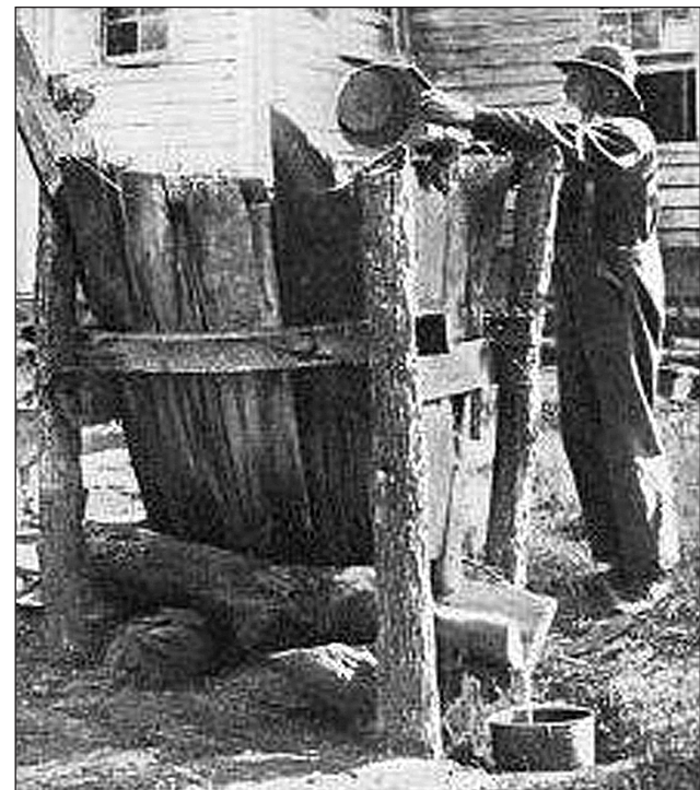
When making soap, colonials would collect hardwood ashes and place them in a hopper, shown above. The hopper was used to separate the lye from the wood ash.
