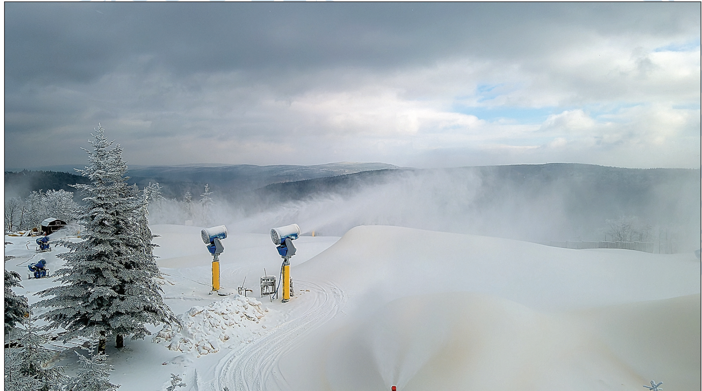
Snow piles up on a slope as the snow guns blast out fresh cover. A mixture of high pressure water and high pressure air join the cold temperature to make snow when the weather isn't cooperating.
