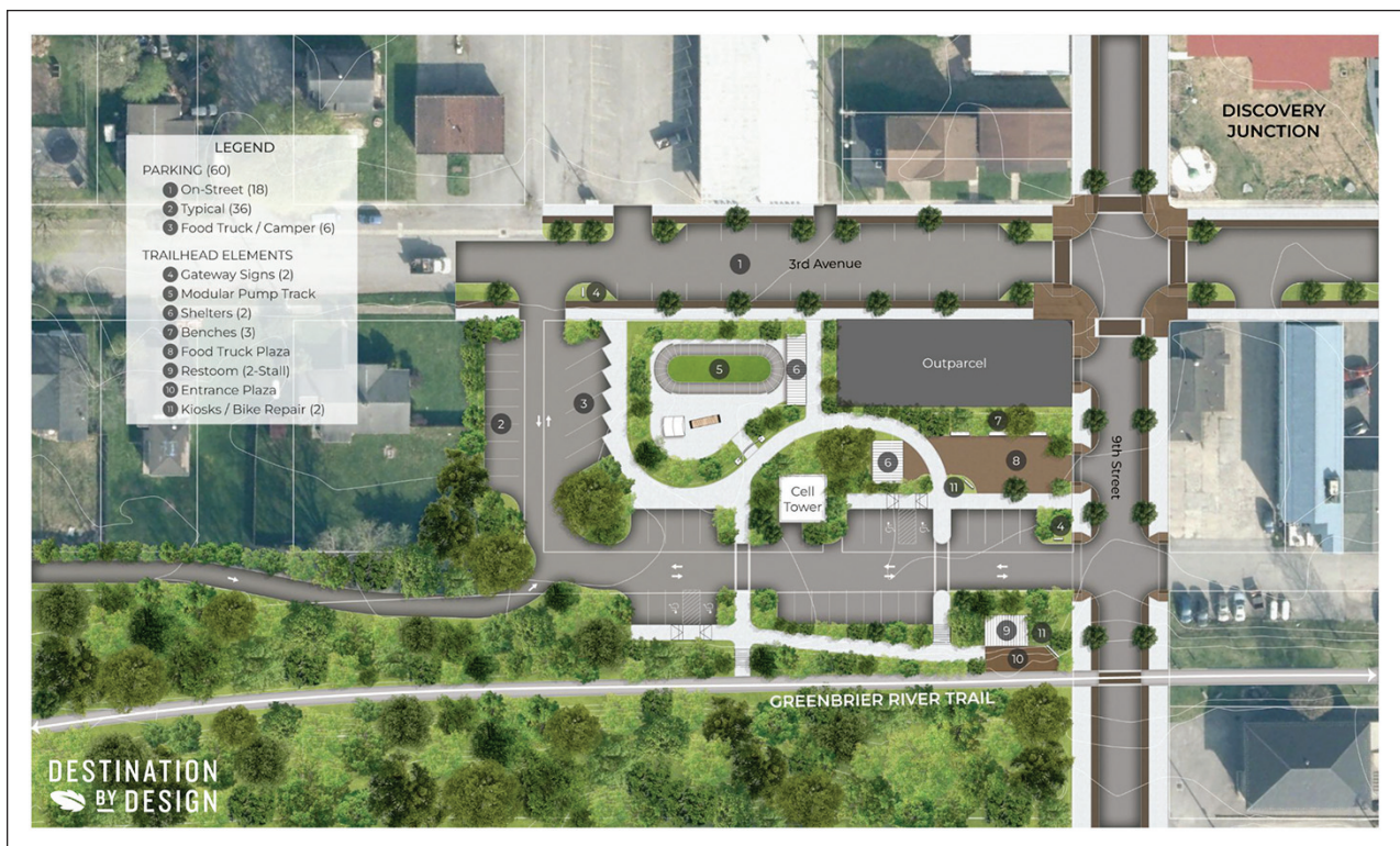
AN ARCHITECTURAL CONCEPT design by Destination by Design in Boone, North Carolina, shows the plan for a trailhead on Third Avenue and Ninth Street in Marlinton. The trailhead will include signage, a pump track, picnic shelters, restrooms and parking for locals and visitors when they use the Greenbrier River Trail or mountain bike.
