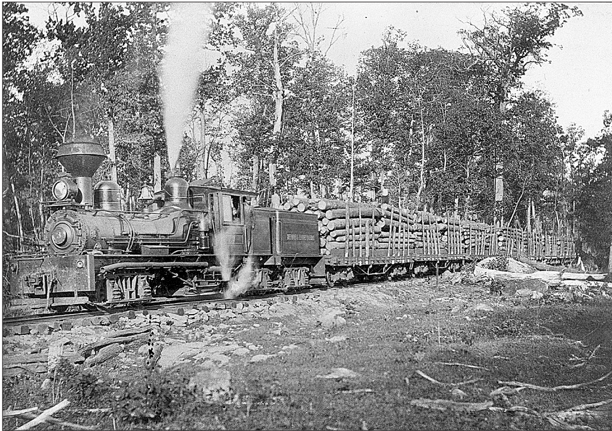
WEST VIRGINIA PULP and Paper Company's Shay No. 3 with nine carloads of logs at the upper switchback on Cheat Mountain near Cass, W.Va. (Pocahontas County Historical Society Collection; ID: PHS000079)
