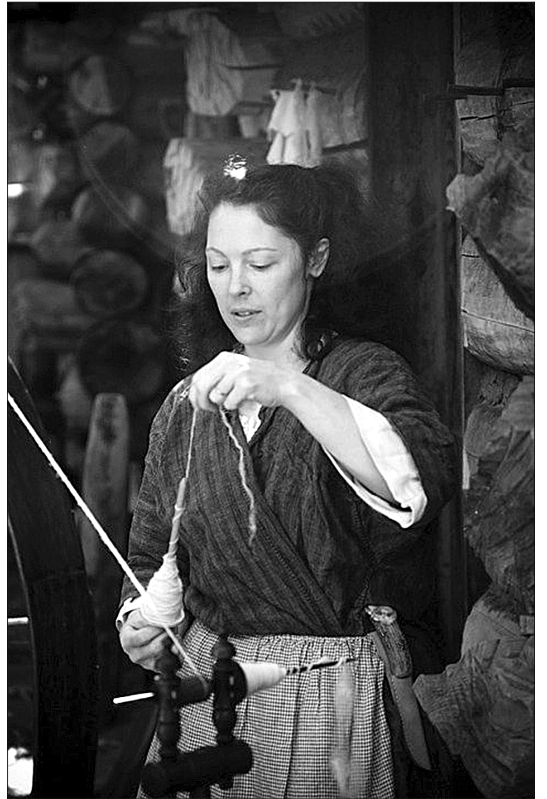
COLONIAL WOMEN SO disrupted the British monopoly on textiles by spinning their own cloth that the Daughters of the American Revolution used the spinning wheel as their organizational symbol. A drop spindle is an easily made tool for spinning wool. The Great Wheel spinning wheel is also referred to as a Walking Wheel due to the back-and-forth walking required while using it.
