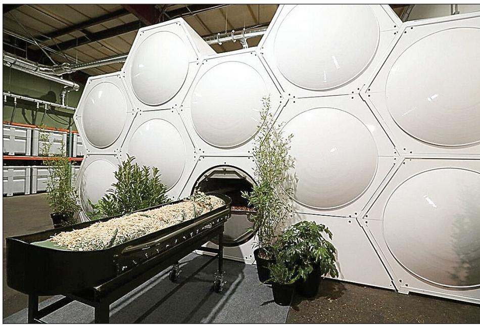
HUMAN COMPOSTING VESSEL ready to enter the composting chamber. Straw, alfalfa, and pine chips are placed on and under the body to ensure enough heat for microbial activity to transform the body into pure, undiluted soil.
