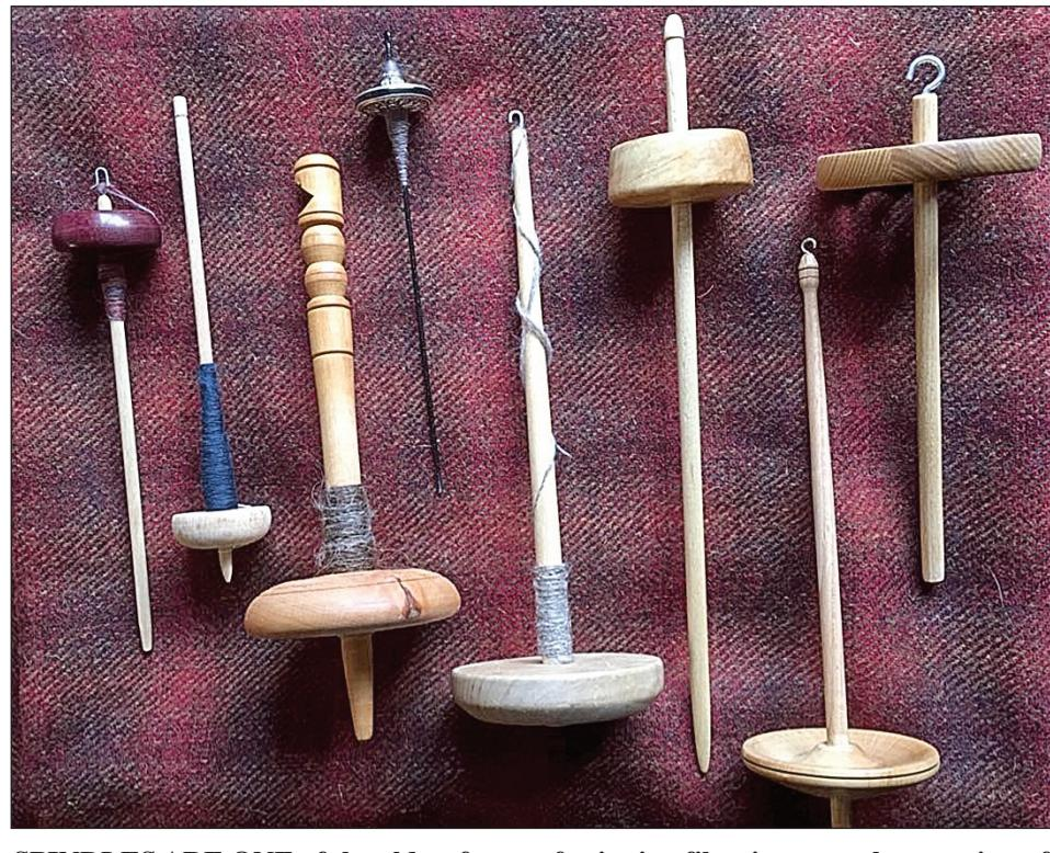
SPINDLES ARE ONE of the oldest forms of spinning fiber into yarn but consists of many more styles and techniques than just the "drop spindle." Photo courtesy of Exarc.net
