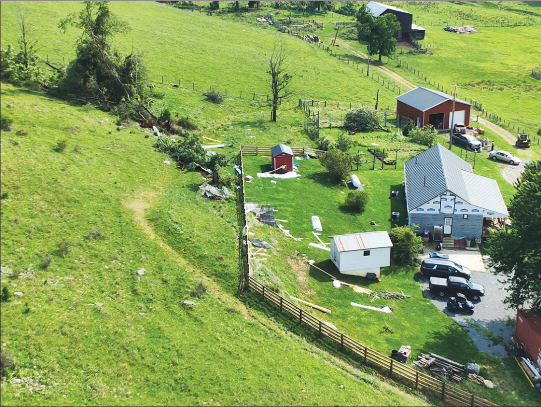
The residence of Brett and Danielle Raines and children is pictured. It shows the debris from their chicken coop structure strung through the yard. Note the storage container in the lower right corner of the photo. The chicken coop was lifted up over that structure as it was strung through the yard. The large tree visible fell in a different azimuth than the trees over along the Troublesome Valley Road.
