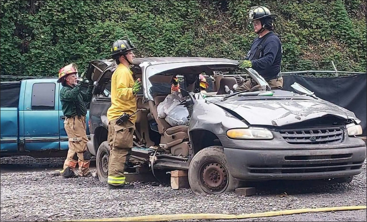
Participants work to remove a minivan’s roof during vehicle extrication training Oct. 3-4 at LJ Recycling. Instructors from Oakwood led the course, which included vehicle stabilization, door and roof removal, and dash rolls (Contributed photo).
