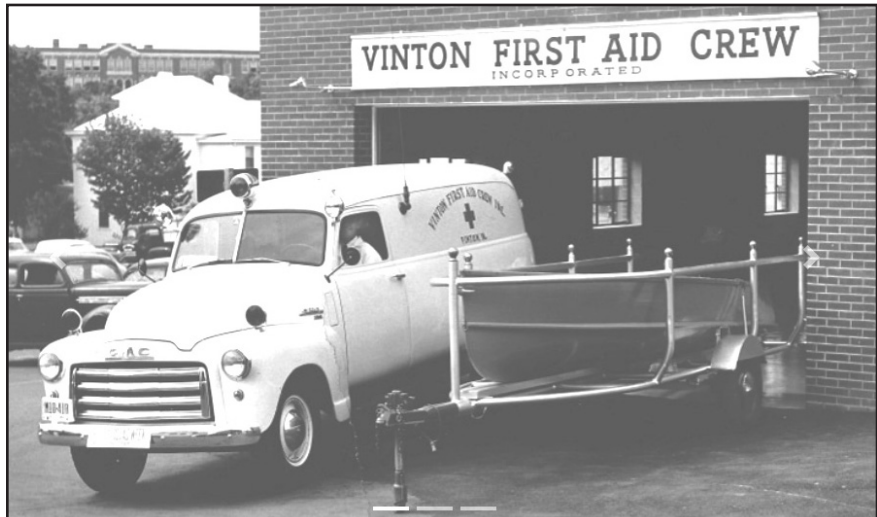
The Vinton First Aid Crew at one time used rescue boats for the Roanoke River and Smith Mountain Lake. This boat trailer was built at the Norfolk & Western shops and later was modified to add a second level for a second boat. The building behind the vehicle is the original First Aid Crew building constructed by volunteers.
