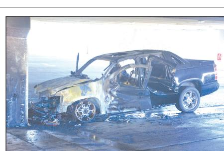
A vehicle parked on the second level of Rosie's parking garage was destroyed by a fire that originated in the engine compartment.
