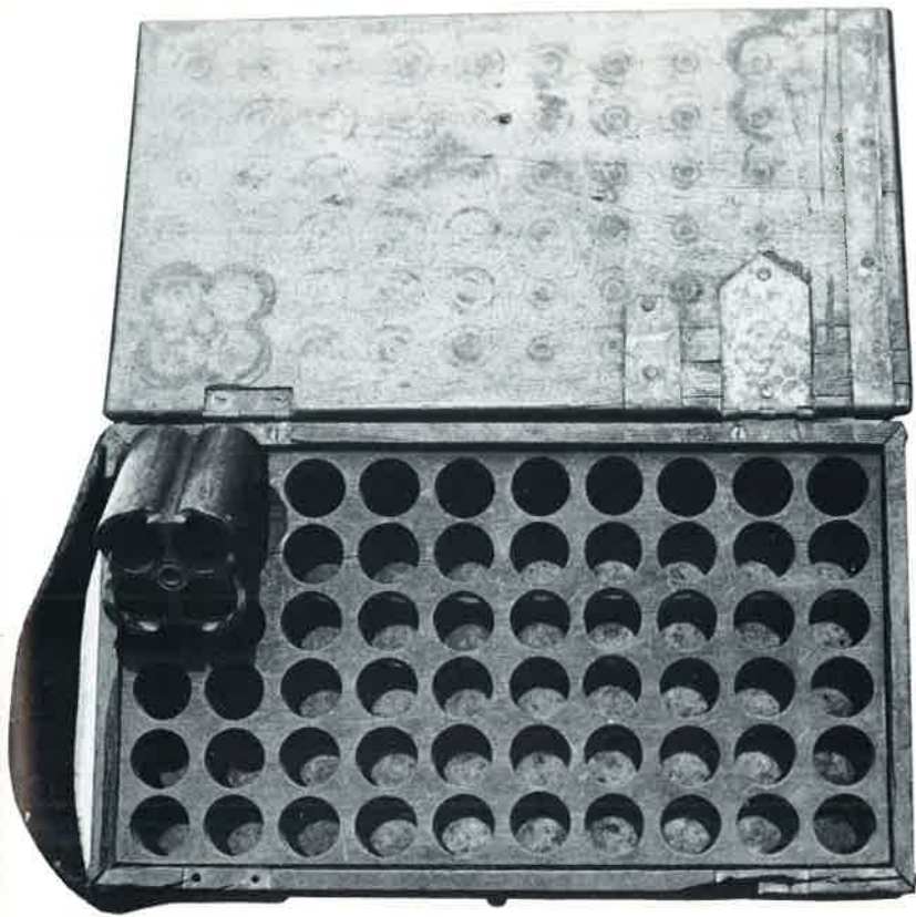
Close up detail of an unmarked cylinder for 4, 12 gauge shotgun shells. Although it is unmarked, the piece is quite close to the patent specifications of Providence gunsmith James A. Crocker's revolving shotgun which, apparently, never went into production.
