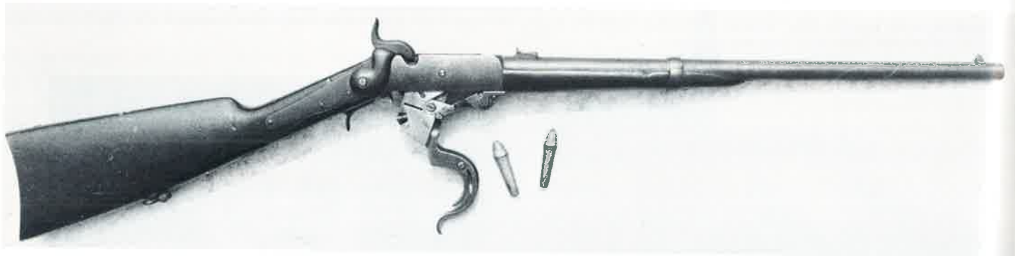
A fourth model carbine with the breech open demonstrating the pivoted block — the patented improvement of Dr. Isaac Hartshorn.
