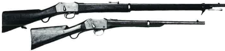
Comparison of the Peabody-Martini B-Model rifle (length - 49 inches) and the carbine (length - 37½ inches).
