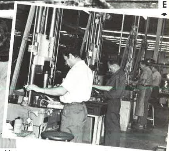
A - Setting diamonds by hand, B - Working on Karat gold ring, C - Designing new item, D - Handcrafting new design, E - "Drop hammers" produce new design in quantity.
