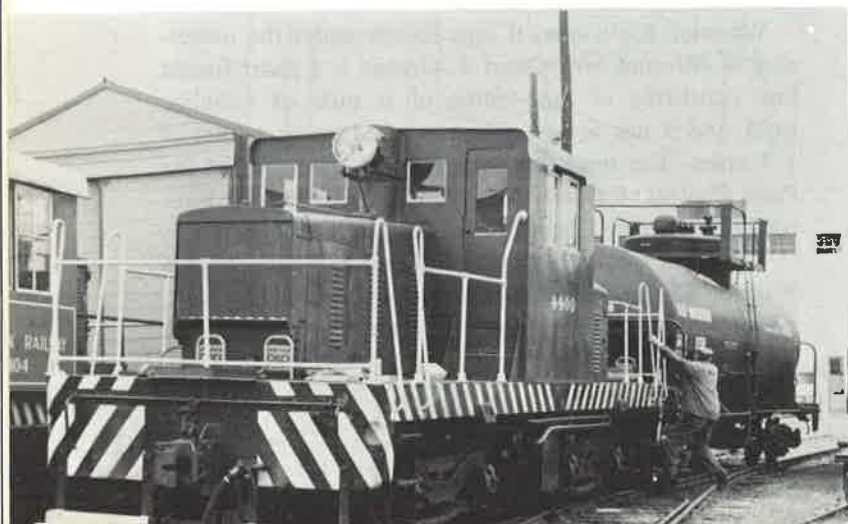
65-ton Vulcan diesel electric locomotive, one of the two "work horses" of the Warwick Railway
