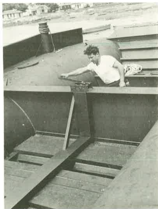
Blount employee is shown testing the hopper section of the RHODOYSTER. Capacity was 70 tons, carried in two seven-foot bins.
