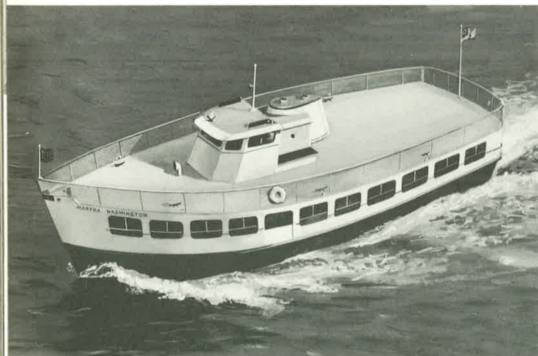
Newest of the Blount 64'6" passenger vessels, the Martha Washington, is designed to carry 350 passengers. (Under construction for the Wilson line of Washington, D. C. when this book went to press).
