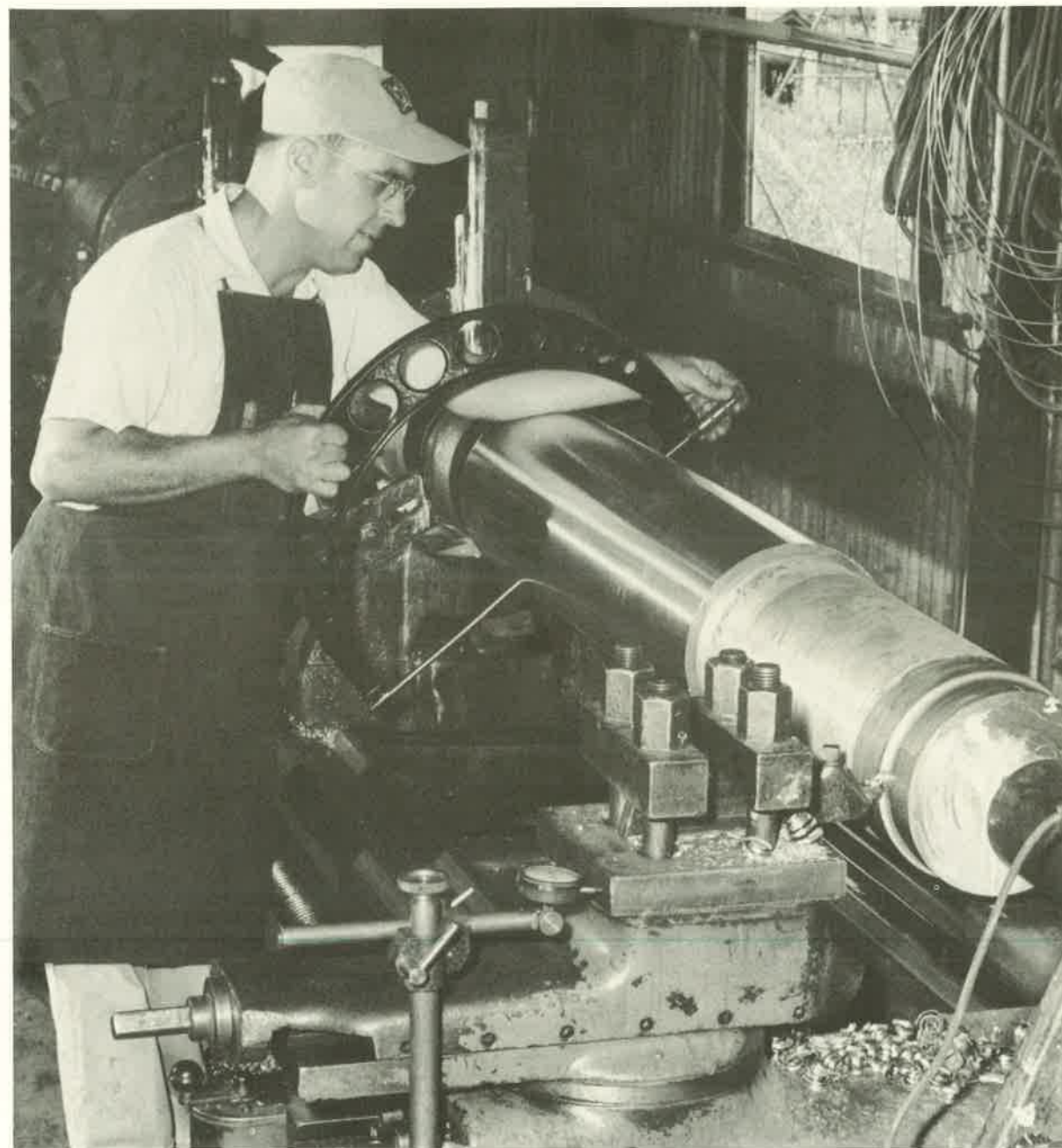
Machinist puts finishing touch on tail shaft. Blount machine shop features a complete range of heavy equipment and skilled machinists.
