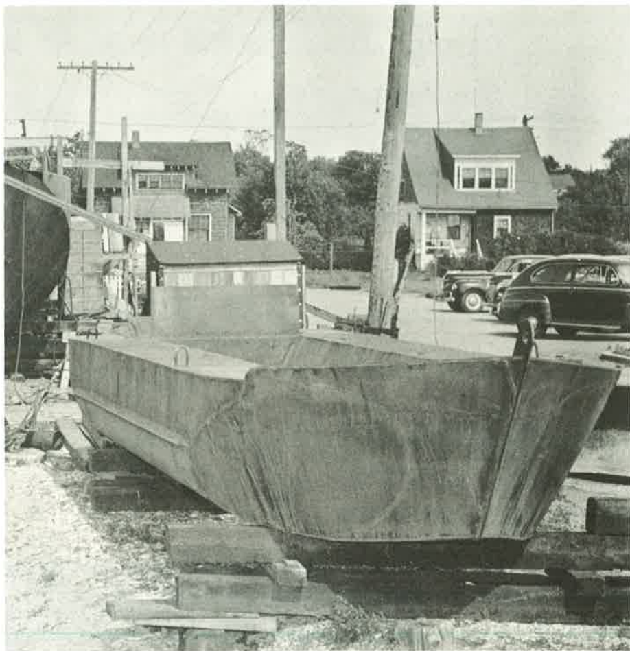
ANNA B Similar to the DEBORAH JUNE, except for smaller dimensions, the ANNA B is also a twintube design, and the fifth vessel built by Blount. She is an oyster cultivator operated
