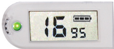
Figure 16 - LCD showing an IOP measurement of 16 and statistical confidence indicator of 95
