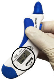
Figure 3 - Tono-Pen AVIA Verification Pass
