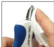
Figure 18 - Wiping Down the Tip
