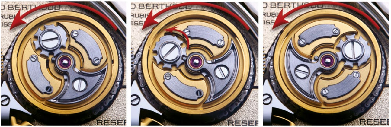
Figure 2: Each rotation brings the Maltese Cross system on the top of the barrel into contact with the pin in the centre, causing the Maltese Cross to take one tooth forward.
