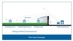
The graphics above show two examples of noise walls located between buildings and a road. In both cases, the wall will shield one of the houses but will not shield them all. Noise walls do not completely eliminate all noise.
