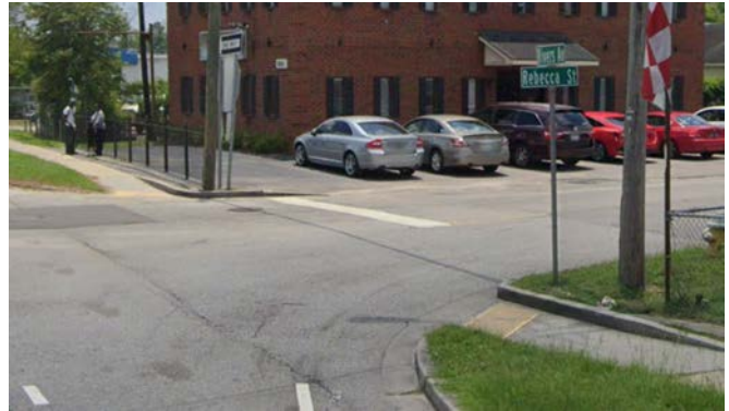
Existing pedestrian facilities on Rivers Avenue (note lack of sidewalks on Rebecca Street and obstacles blocking off-street access to Rivers Avenue sidewalk)
