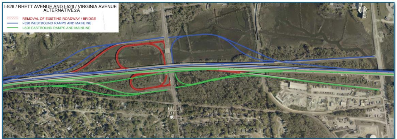
Figure 1.6: Proposed Interchange Configuration at North Rhett and Virginia Avenue in North Charleston
