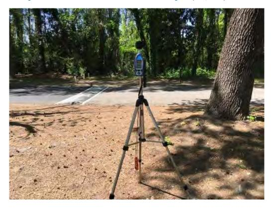
Figure A.12. I-526 WEST – Ambient Noise Monitoring Setup 5C, Receptor 5C
