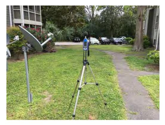
Figure A.15. I-526 WEST – Ambient Noise Monitoring Setup 6A, Receptor 6A-a
