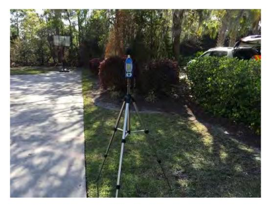
Figure A.23. I-526 WEST – Ambient Noise Monitoring Setup 9, Receptor 9a
