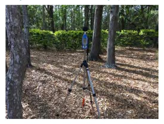
Figure A.24. I-526 WEST – Ambient Noise Monitoring Setup 10, Receptor 10
