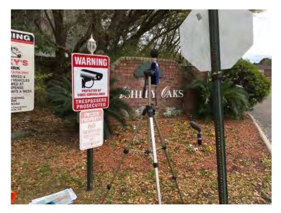
Figure A.19. I-526 WEST – Ambient Noise Monitoring Setup 7, Receptor 7a
