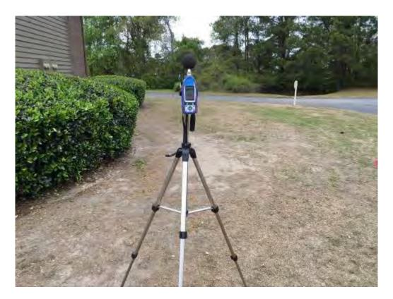
Figure A.11. I-526 WEST – Ambient Noise Monitoring Setup 5B, Receptor 5B-a
