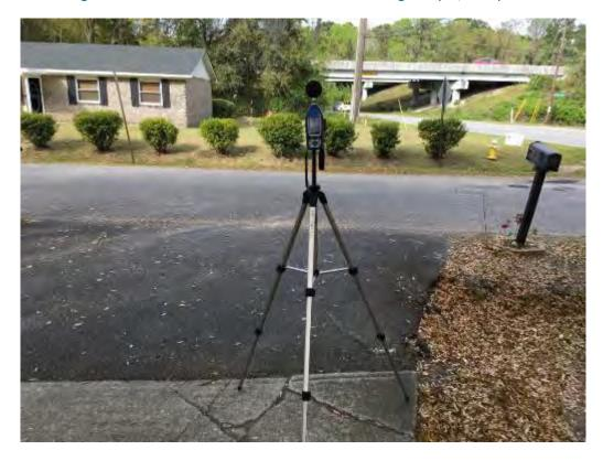
Figure A.4. I-526 WEST – Ambient Noise Monitoring Setup 2, Receptor 2a
