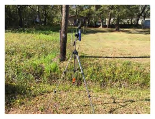
Figure A.40. I-526 WEST – Ambient Noise Monitoring Setup 26A, Receptor 26A
