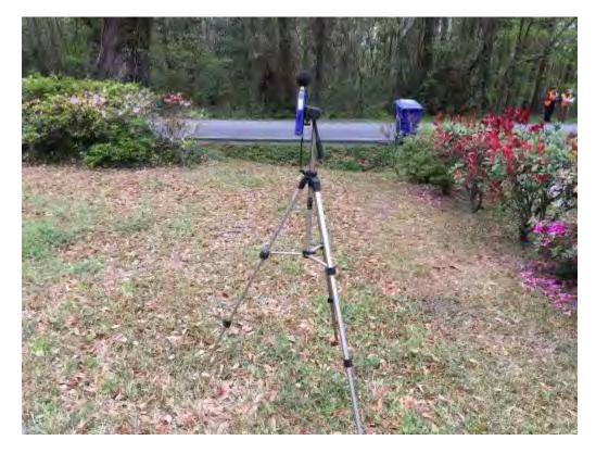
Figure A.2. I-526 WEST – Ambient Noise Monitoring Setup 1, Receptor 1a
